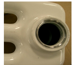
Left hand thread not marked
